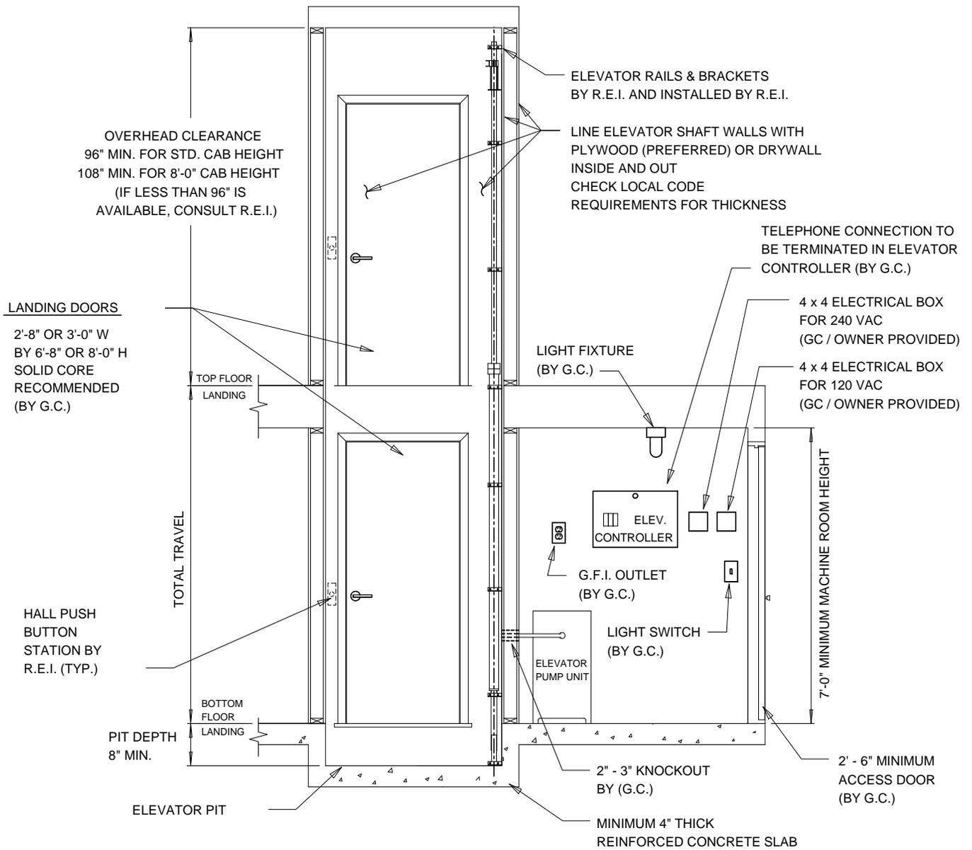
RESIDENTIAL ELEVATORS (REI) CONTROL SYSTEM CONTAINS THE 240 VAC AND 120 VAC DISCONNECTS, HOWEVER; GC/ OWNER MUST PROVIDE DEDICATED CIRCUIT AND WIRE TO 4" x 4" BOX (1 FOR 240 VAC & 1 FOR 120 VAC) IN MACHINE SPACE PER DRAWING. SEE REI ELECTRICAL REQUIREMENTS BROCHURE FOR FURTHER DETAILS.
